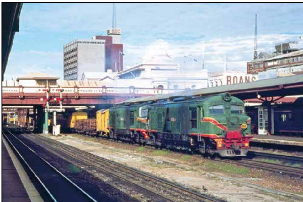
Above left: The X type locomotives were known to have the occasional on board fire during their operational lives. Some type of issue seems to have arisen with XA1405 working 44 goods at Waroona on Saturday 30 May 1970, a visit to the roof area with a fire extinguisher being required.
